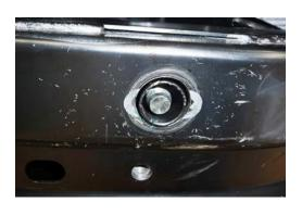
9. Reinstall mounting cradle to vehicle, centralise, insert and tighten all mounting harware.
