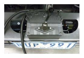
4. Connect three colour coded cables to the corresponding poles on winch motor.
