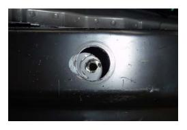
6. Open the inner holes to 12mm
