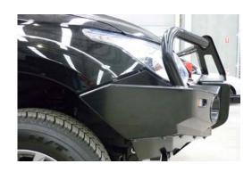
16. Once bull bar is aligned with vehicle and bolts tightened, drill through pinning holes (circled in yellow) between bull bar and chassis bracket and secure with bolts, washers and nuts provided.
